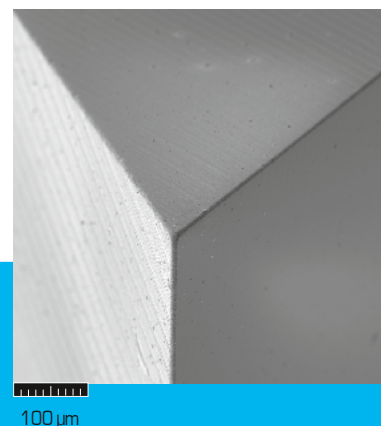
DLC3 coated endmill under scanning electron microscope:
