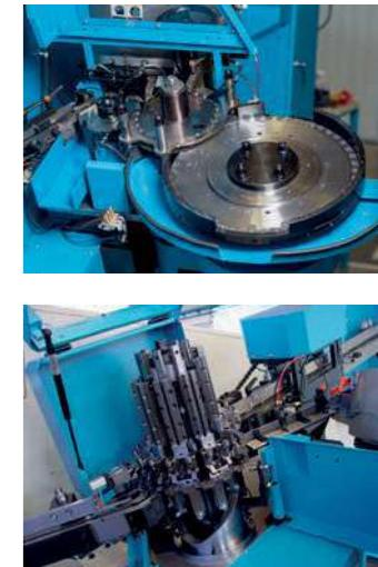
This machine incorporates a system for inserting washers into the parts before rolling.
