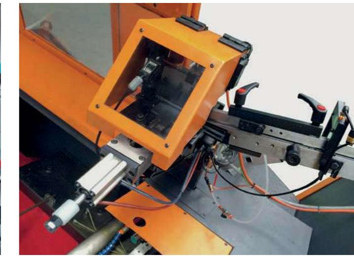
This machine incorporates a feeding system for headless parts into a rolling machine.
