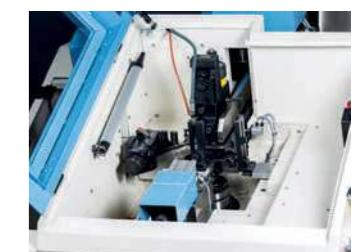
**These are secondary operation machines for the fastener industry in which their main function is the facing and chamfering of parts, their flexibility allows numerous operations.**
