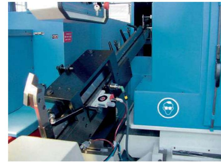
**They are long stroke rolling machines specially designed for the forming of complex profiles.**
